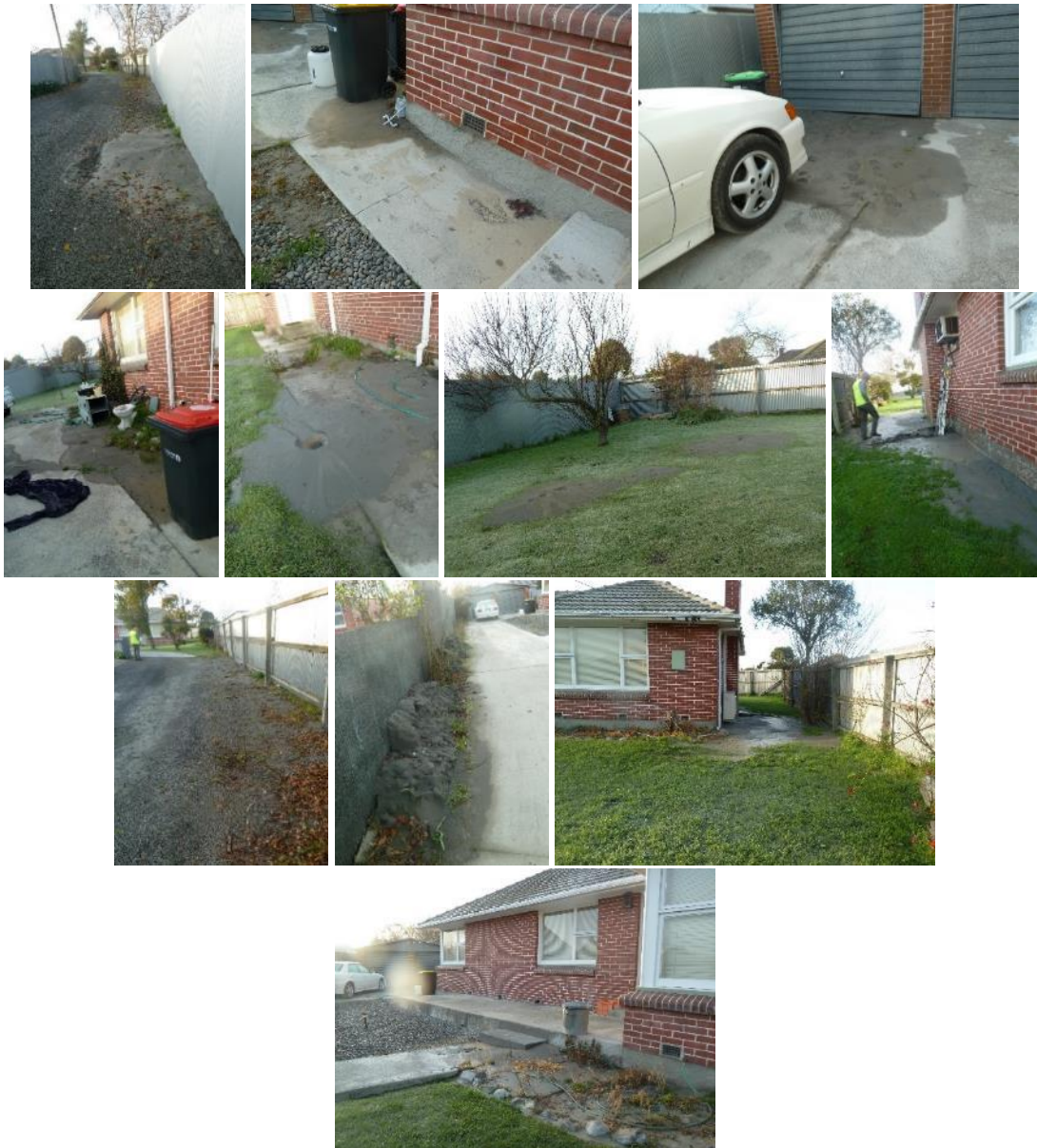
Figure 78: Ground photographs showing ejecta at the property with Patch B (photograph date: 17 June 2011).
