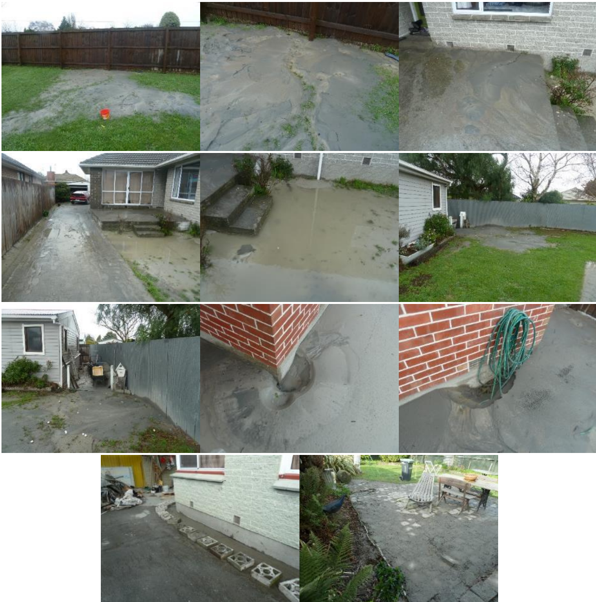
Figure 82: Ground photographs showing ejecta at some properties within the 50-m buffer (photograph date: 17 June 2011).
